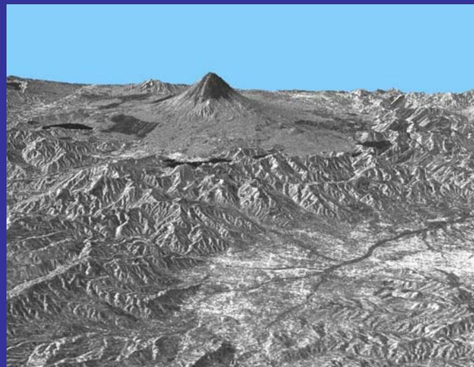
Mt. Fuji's terrain elevation map derived by JERS-1/SAR stereo.
