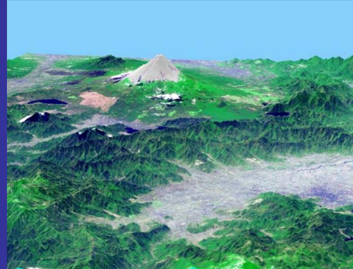
Mt. Fuji's terrain elevation map derived by JERS-1/OPS stereo.
