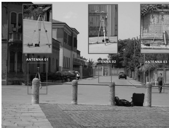
Figure 7. The three antennas in the scanner's field of view
