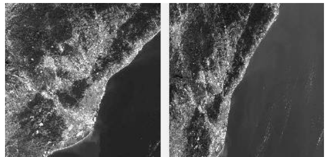
Figure 2: THR image (left, GSD: 2.5m x 2.5m) and HRS1 image (right, GSD: 10m x 5m)
