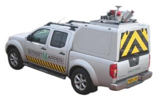
To obtain accurate 3D models for building facades and looking into road conditions, IGI and the British firm 3D Laser Mapping joined forces to build a mobile LiDAR system, *StreetMapper*. *StreetMapper* links laser and camera technology with a high-precision positioning system, *TERRAcontrol*.
