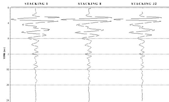
Fig. 7. 1GHz A-scans with different stacking values.
