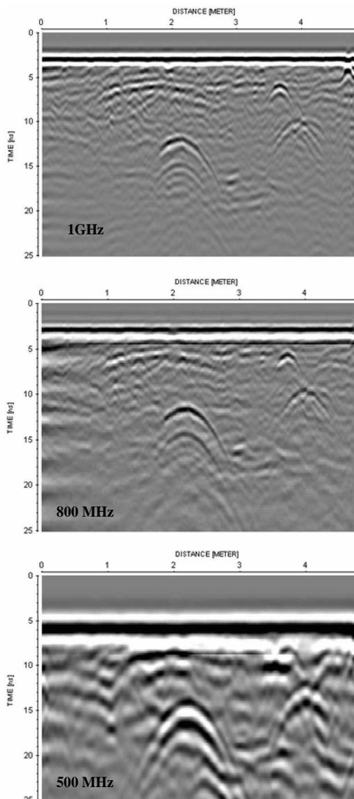
Fig. 8. Example of GPR data obtained on a test site where PVC and concrete pipes of different sizes were present.
