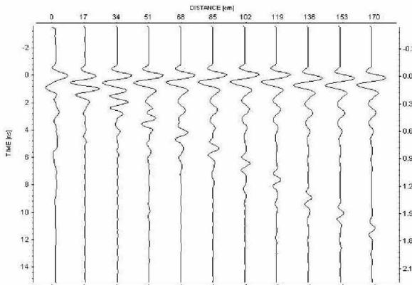
Fig. 5. Sequence of stacked traces for different distances with the 800 MHz antenna
