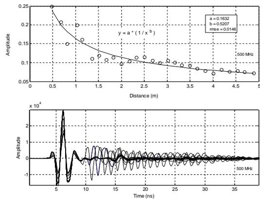
Fig. 6. Results obtained for the 500 MHz antenna.
