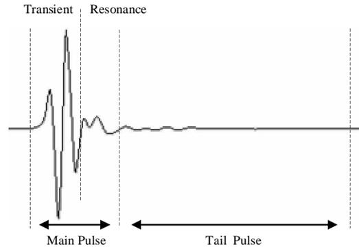
Fig. 2. Time domain 500 Mhz antenna response
