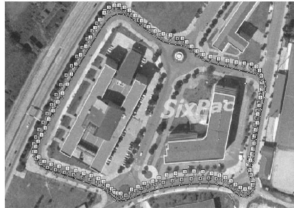
Fig.4. Example of evaluation tests: precision and coordination of available GPS equipment and GPR.
