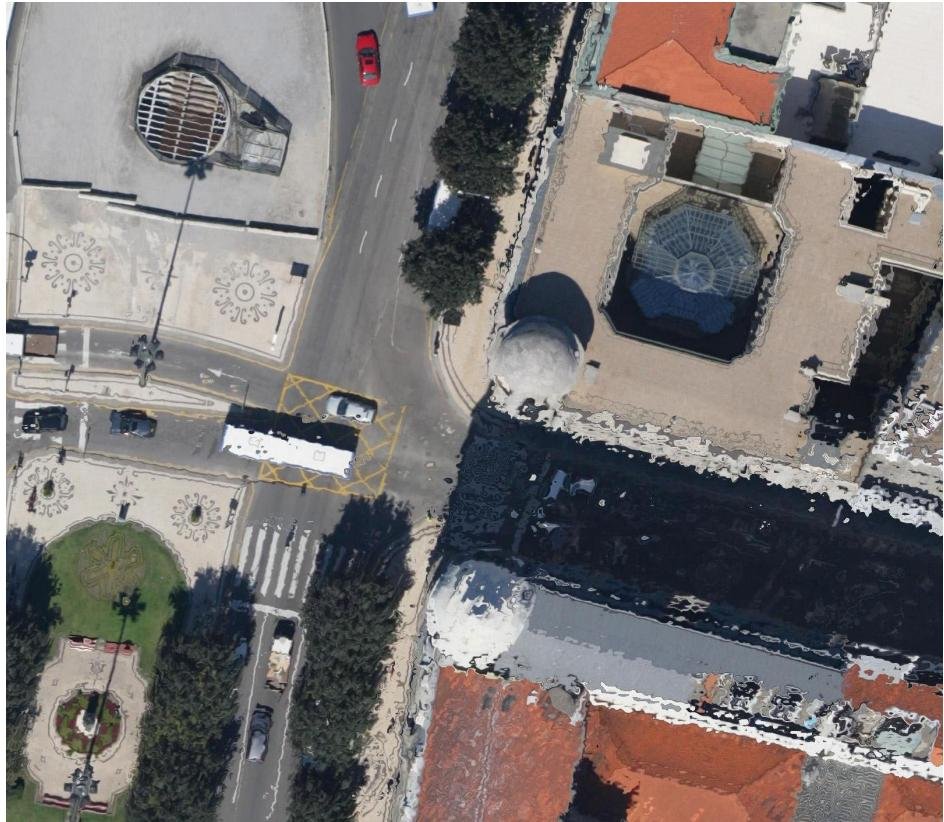
Figure 4 – Orthophoto with blurring effect.
