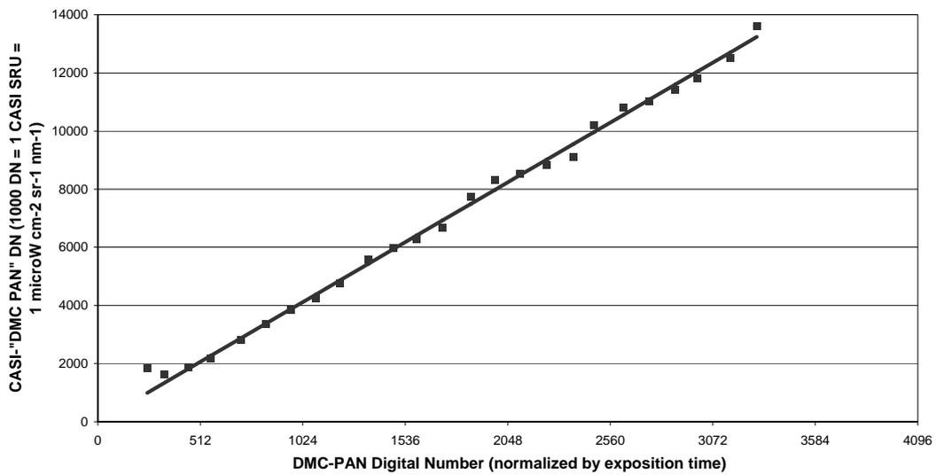
Figure 4.3.1 DMC-PAN Calibration Plot for Fstop 16 with DMC-PAN-like band from CASI images.
