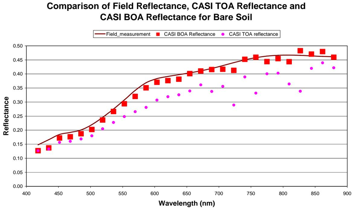
Figure 4.2.1 Comparison of field reflectance, CASI TOA reflectance and CASI BOA Reflectance for bare soil on Banyoles area.
