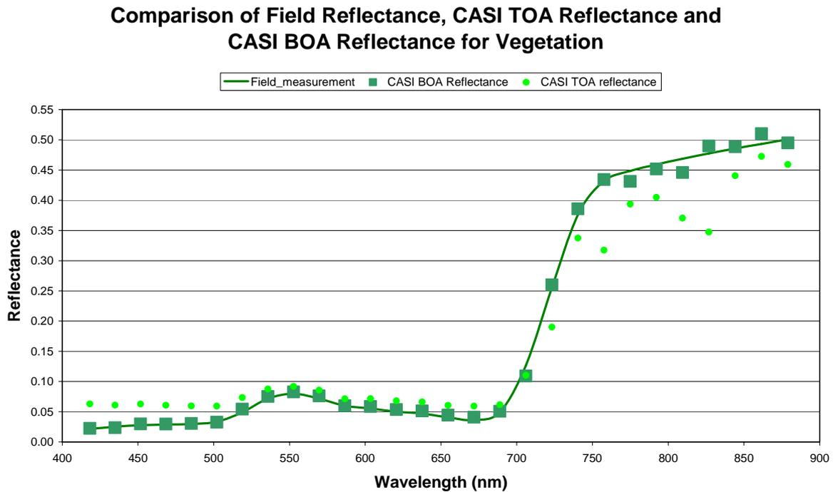
Figure 4.2.4 Comparison of field reflectance, CASI TOA reflectance and CASI BOA Reflectance for vegetation on Banyoles area.
