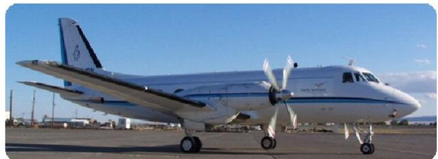
Figure 6. 4STAR mounted in DOE Gulfstream G1 (atop aircraft just ahead of propeller)
