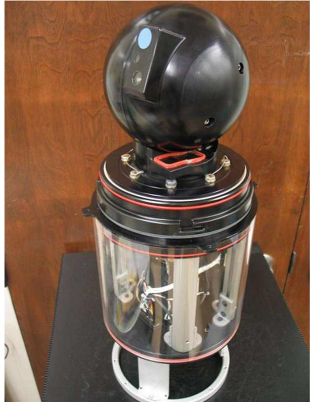
Figure 5. 4STAR flight instrument
