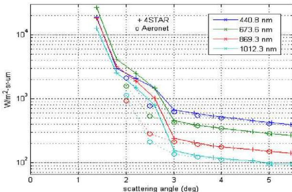
Figure 4. Direct beam contamination of sky light signal close to the sun.
