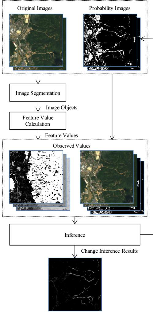
Figure 1 Flow diagram of the change detection approach in this paper.
