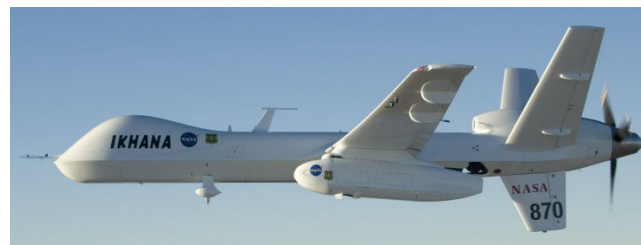
Figure 1. The NASA Ikhana UAS platform. The sensor is carried in a pod located under the wing, as can be seen in this image.
