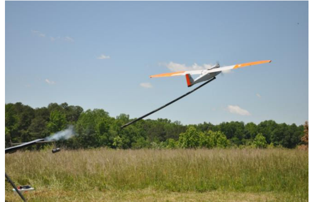
Figure 5. AAI RS-16 catapult-launched (belly-recovered) small UAS employed by USFS in 2010 during a capabilities demonstration to support wildfire imaging. The USFS has organized and supported a series of these capabilities missions to look towards small UAS wildfire observation operations.
