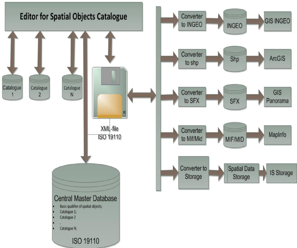
Figure 2. Scheme showing automated preparation of catalogues and qualifiers
