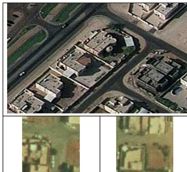
Figure 12: above GeoEye-1 image with 0.5m GSD, below samples from aerial photos with 0.7m GSD
