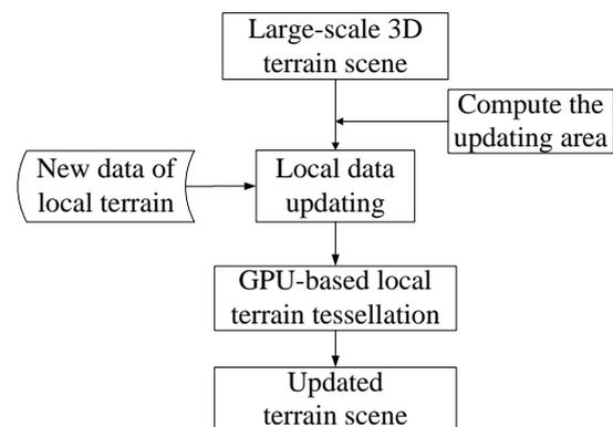
Figure 1. Flow chart of local terrain data updating
