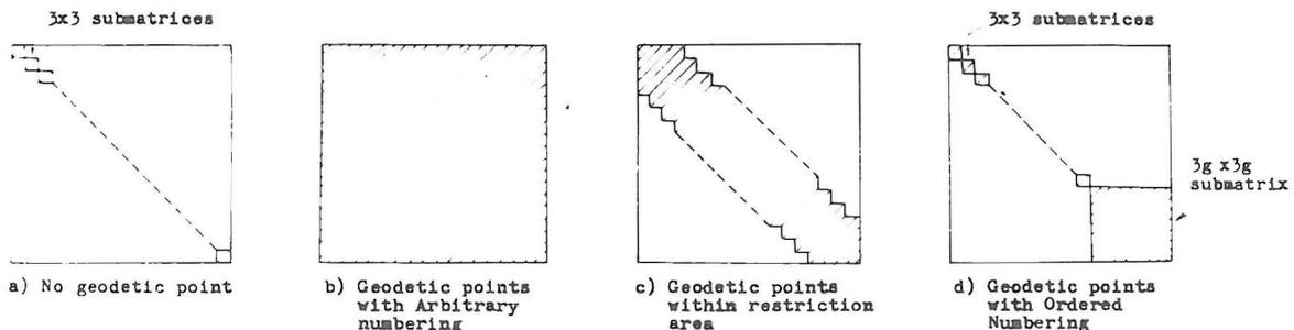
Fig.2 Structure of matrix  $H = H_f + H_g$
