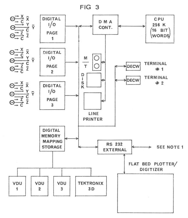
NOTE 1: 9600 BAND TO FLATBED PLOTTER 9600 BAND TO WILD TA TABLE/PRIL CONT. 9600 BAND TO ANALYTICAL PLOTTER 1200 BAND TO TELECOM/TRANSIT LINES 300 BAND TO OLIVETTI TC480 AND/OR CASSETTES
