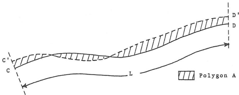
Fig. 4: The area method to evaluate the planimetric accuracy.
