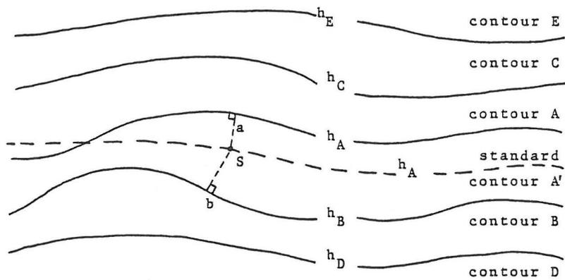
Fig. 1: Point  $S$  is a point of the standard contour  $A'$  at which the height is interpreted from the participant's data.
