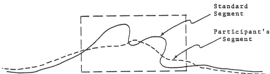
Fig. 7: Generalization of a participant's data due to the relatively smaller scale used causes the Point Method to overestimate the errors calculated. The generalization is illustrated in the dashed rectangle.
