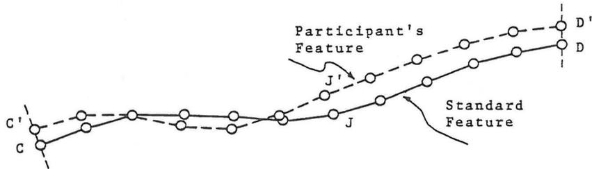
Fig. 5: The Generated Point Method to evaluate the planimetric accuracy.
