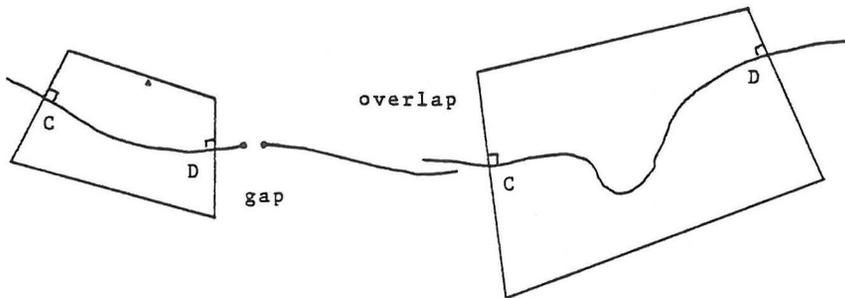
Fig. 6: Standard segments are selected using a window with two sides approximately perpendicular to the feature at the end points C and D. Visible gaps and overlaps were excluded.
