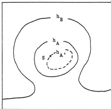
Fig. 3: Contour  $h_{A'}$  will be eliminated from the test. The entire  $h_{A'}$  is enclosed by a participant's contour and therefore its height can only be extrapolated.
