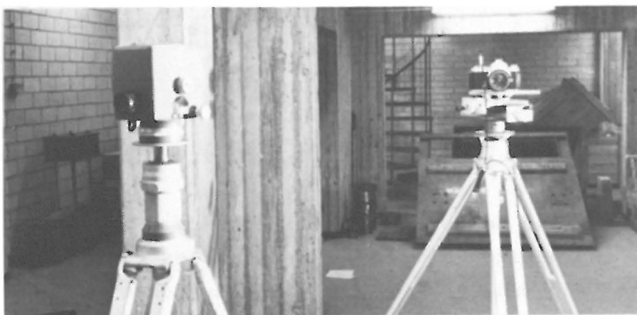
Fig. 4. Measuring the height of perspective center.
