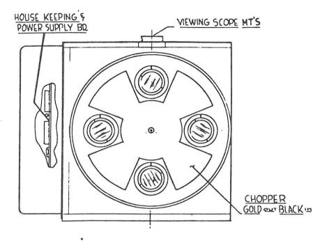
Figure 8. Chopping arrangement for the multiband radiometer.
