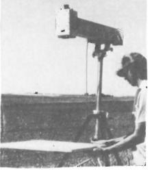
Figure 4. Tripod platform for Landsat band radiometer.
