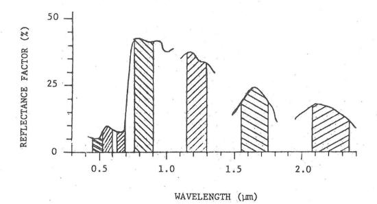
Figure 6. Spectral distribution of passbands superimposed on a typical vegetation spectrum.
