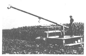
Figure 3. Pick-up truck mounted boom platform for Landsat band radiometer.
