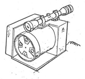
To achieve reliability in reflectance measurement, a field calibration procedure using a reference surface is to be employed for the reflective spectral bands.<sup>10</sup> For the thermal channel, direct field comparison with two reference blackbodies at known temperature will be used to establish the thermal radiance scale.
