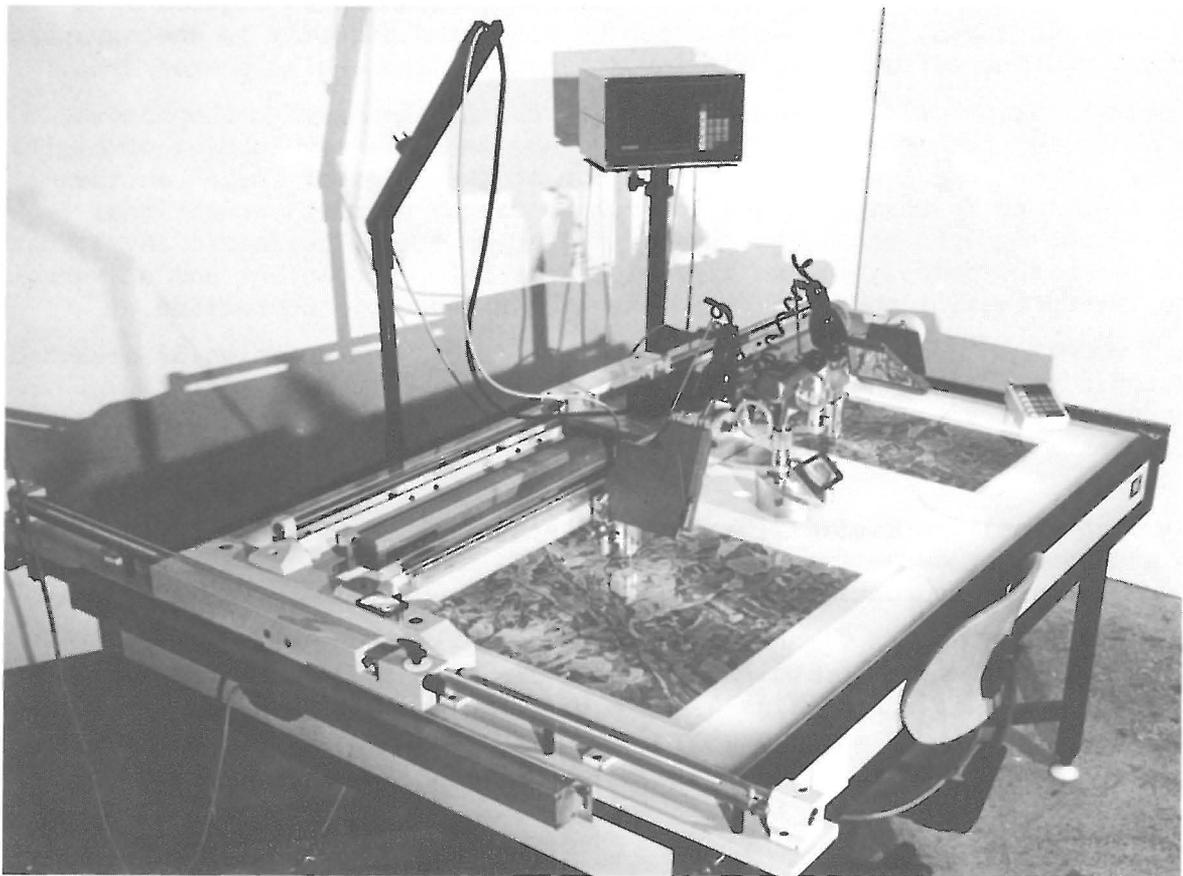
*Fig. 2: STEREOGRAPH when compiling stereo-orthophotos*
