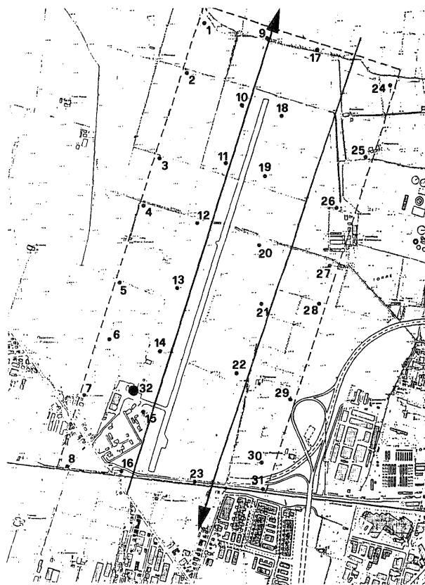
Figure 2.1 - Parma experiment: testfield configuration and photogrammetric project.
