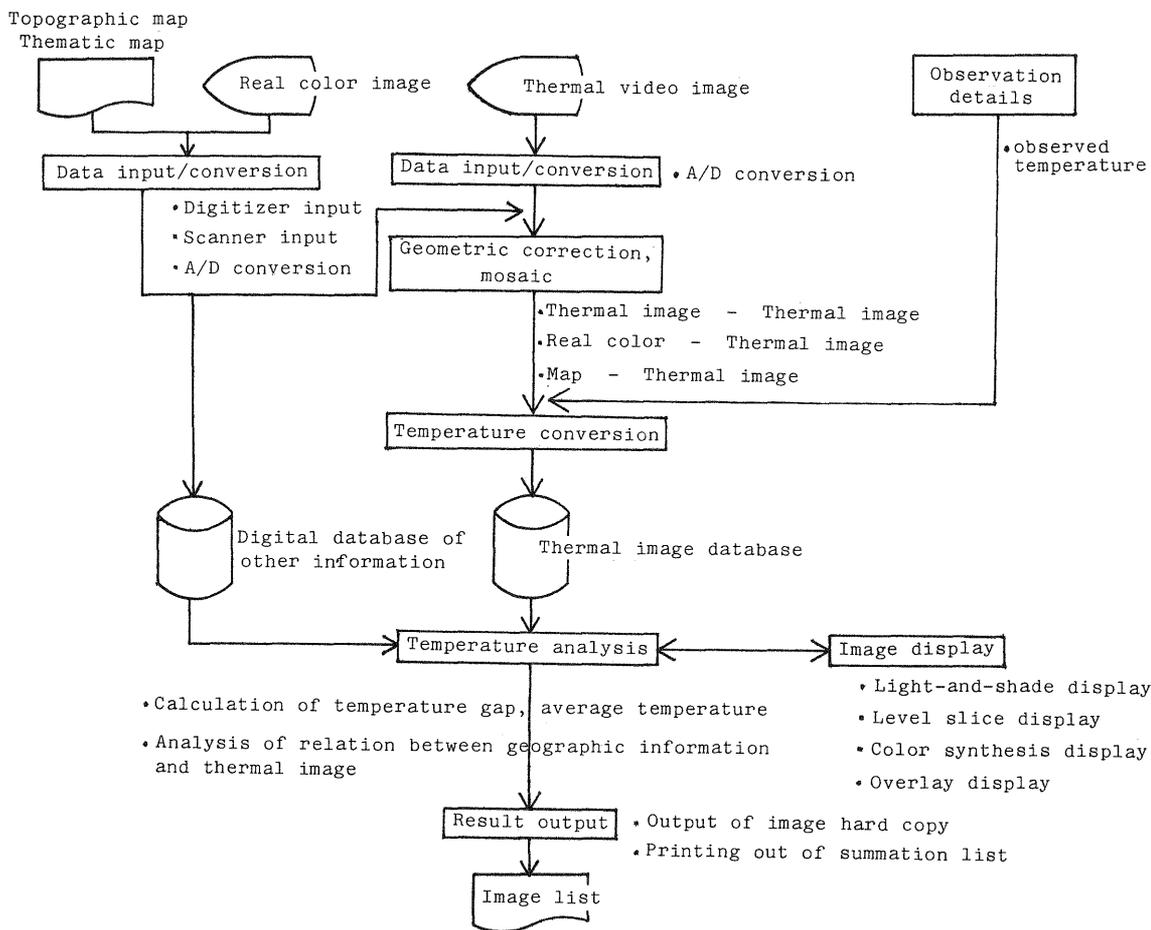
Fig. 7 Flow of processing
