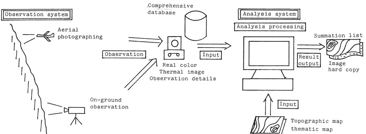
Fig. 1 Diagram of system configuration
