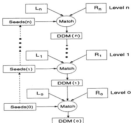
Figure 4: Multi-Resolution Stereo Matching
