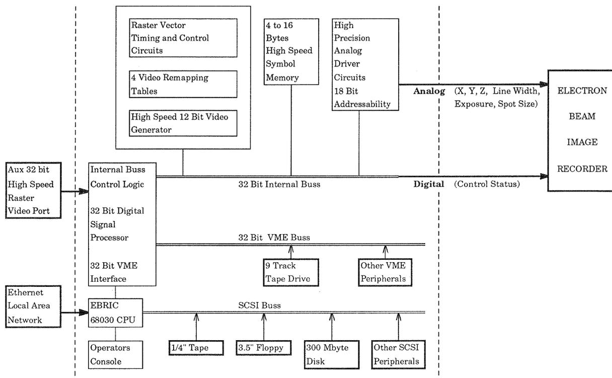
Figure 2 Block Diagram of RVG 450
