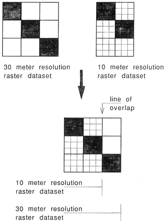
Figure 3 Mosaicing with Different Cell Sizes (Data Fusion)
