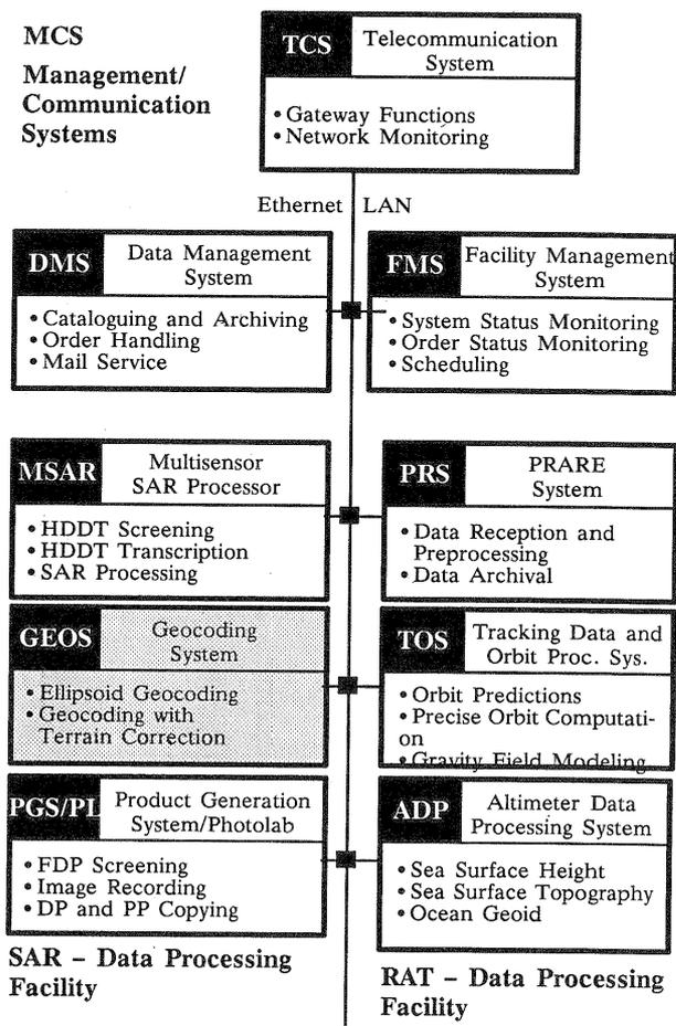
Figure 1: German Processing and Archiving Facility for ERS-1 (D-PAF)
