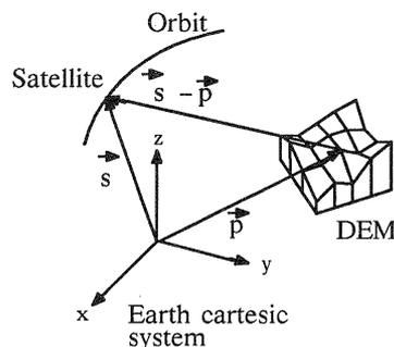
Figure 2: Satellite SAR Geometrie
