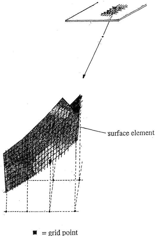
Fig.3 Projection of the image densities onto the surface
