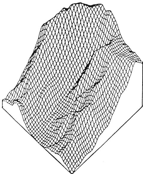
Fig.1 Surface registration by a regular and dense point grid
