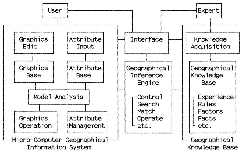
Fig. 3 The structure of MCGES
