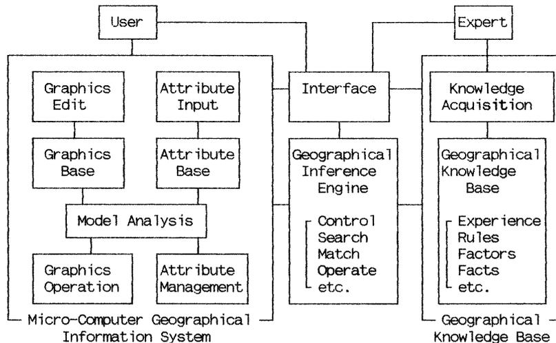
Fig. 3 The structure of MCGES
