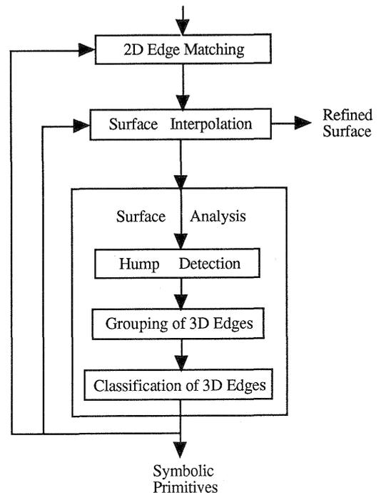
Figure 1. 3D urban area surface analysis module
