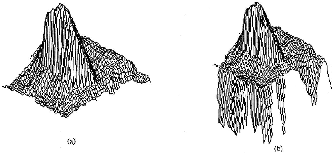
Figure 4. Classification examples. (a) Top of the library in Figure 3(e) generated by only the horizontal edges which are above the topographic surface. (b) An incomplete library generated by vertical edges and horizontal edges which are above the topographic surface.
