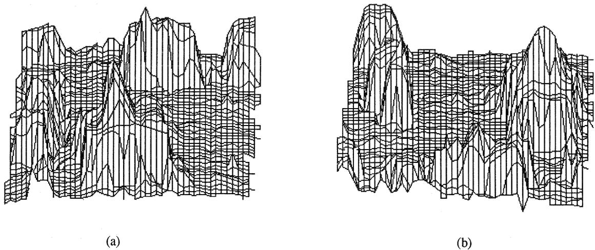
Figure 5. The re-interpolated DEM surface. (a) and (b) Two view angles of the re-interpolated DEM surface. The building walls in this figure are more vertical than those in Figure 2(c).
