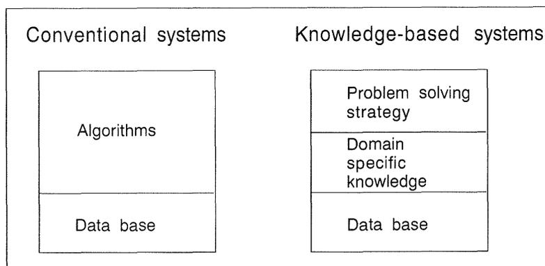
Figure 4 : Conventional versus knowledge-based systems architecture.
