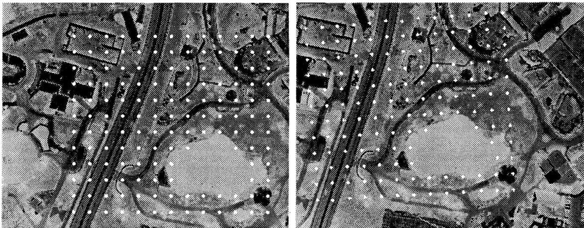
Figure 13: Matching results with a 72 pixel interval on a stereo pair captured by a high resolution CCD camera.
