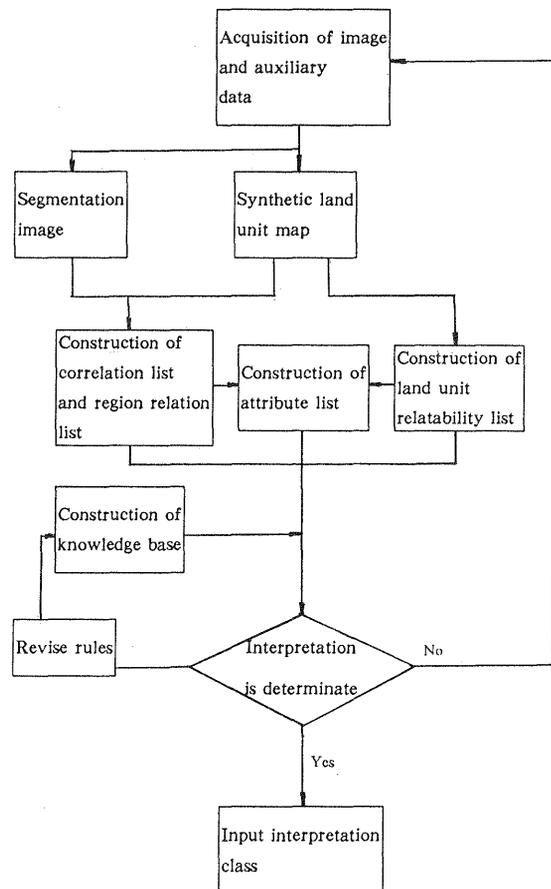
Figure 6. A procedure to interpret an image based on multilevel representation tree.
