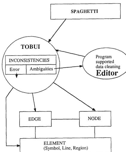
Fig 3: Data flow in the Topology Builder
