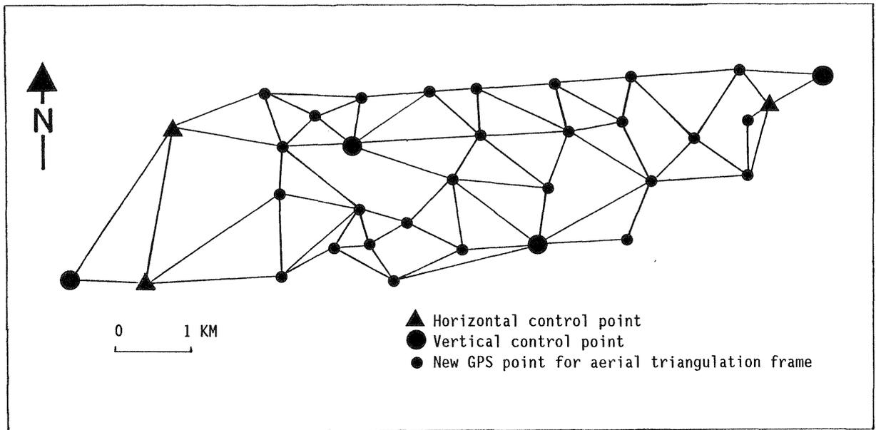
Figure 2. GPS frame for aerial triangulation, controlling an engineering project.
