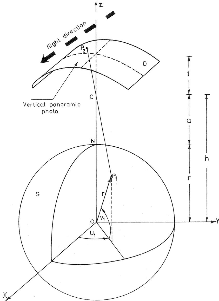
Fig.1. Geometry of a panoramic photograph.
