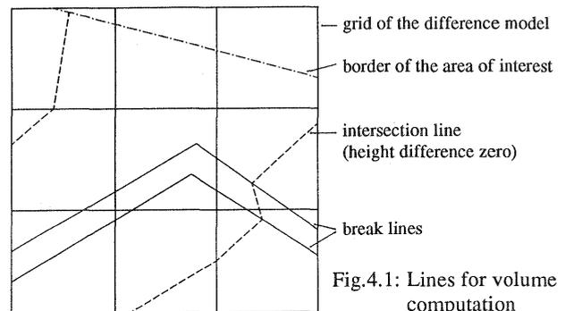
Fig.4.1: Lines for volume computation
