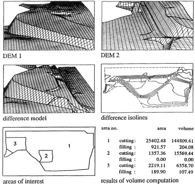
Fig. 3: Example of a volume computation
