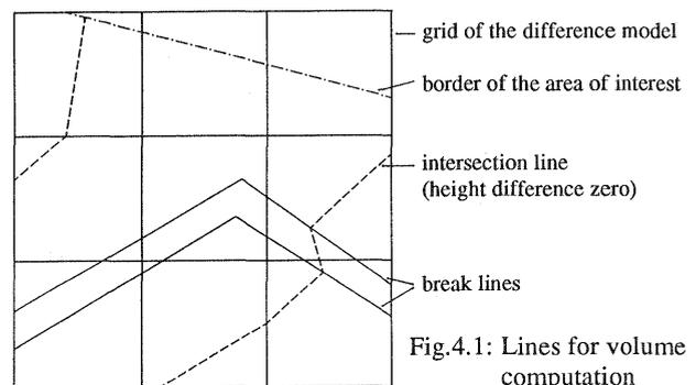
Fig.4.1: Lines for volume computation
