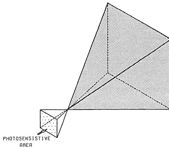
Figure 4 Volume of Space Viewed by Area Array Sensors
