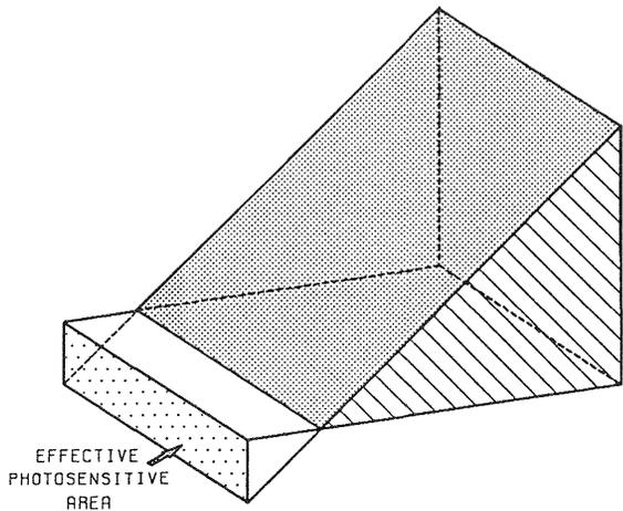
Figure 5 Volume of Space Viewed by Line-Scan Sensors
