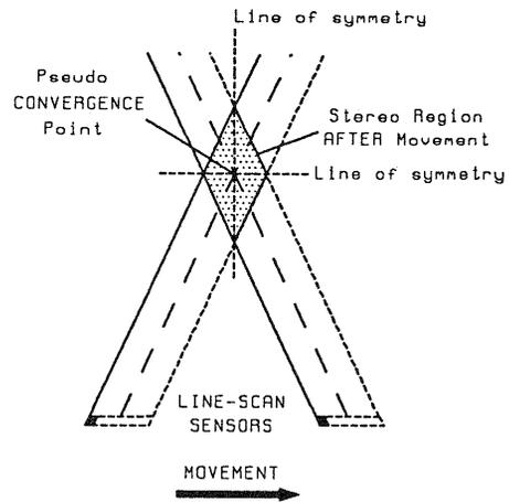
Figure 12 Stereo Region for Lateral Motion Line-Scan Sensors
