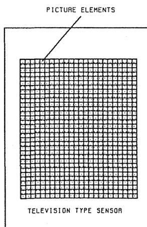
Figure 1 Photosensitive Area of Television Type Sensor
