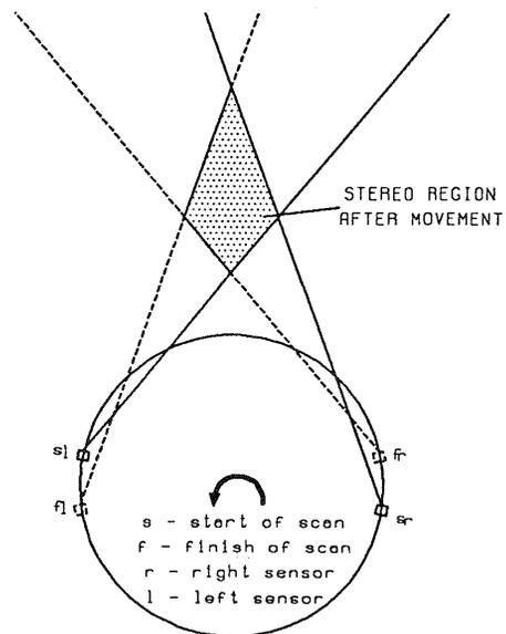
Figure 13 Stereo Region for Rotational Motion Line-Scan Sensors
