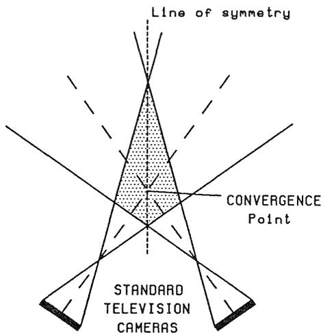
Figure 11 Stereo Region for Television Type Sensors
