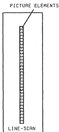
Figure 2 Photosensitive Area of Line-Scan Sensor
