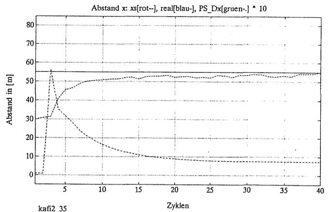
Figure 8b Estimated distance with a reduced measurement vector due to occlusion
