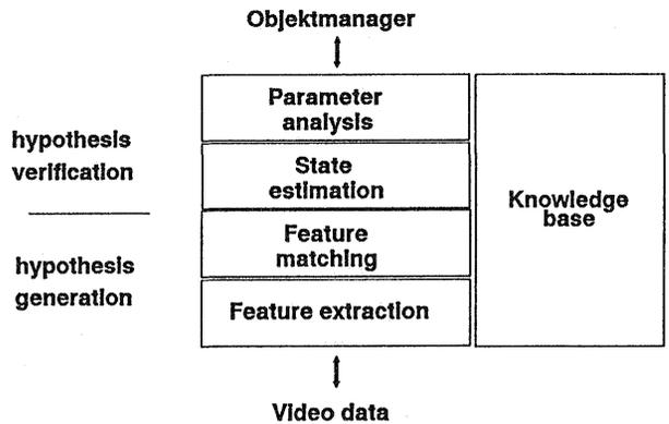
Figure 6 Components for recognizing occluded objects
