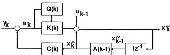
Figure 7 Recursive estimation by a Kalman filter scheme
