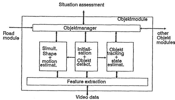
Figure 2 Structure of the object recognition module
