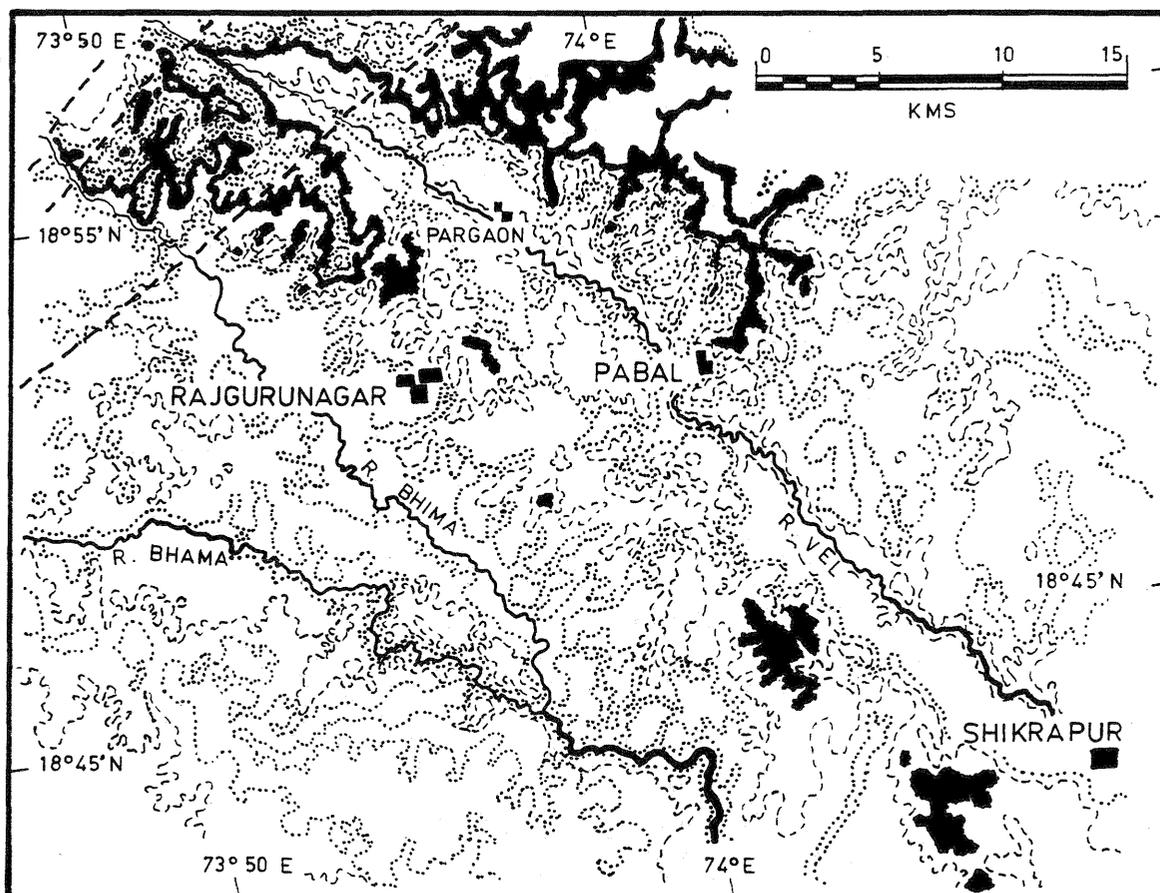
FIG.5(B) : Flow map of the Pabal - Rajgurunagar area (around 30 km north of Pune), based on the visual interpretation of the LISS-2 and TM data as in 5(A).
