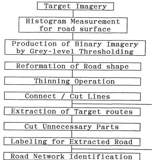
Fig.5 The procedure for Road Network Extraction
