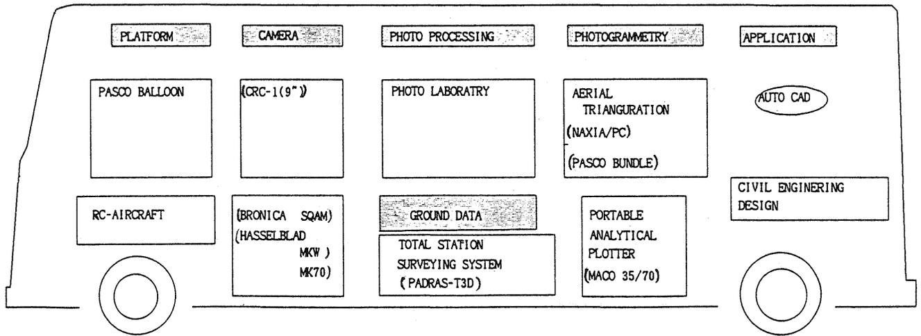
Fig.1 PADRAS CAR System-"Patent applied for".
