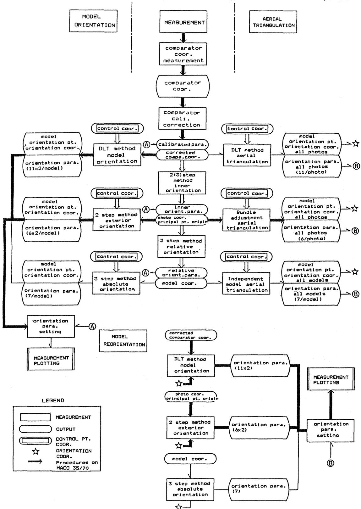
Fig.2 Orientation process
