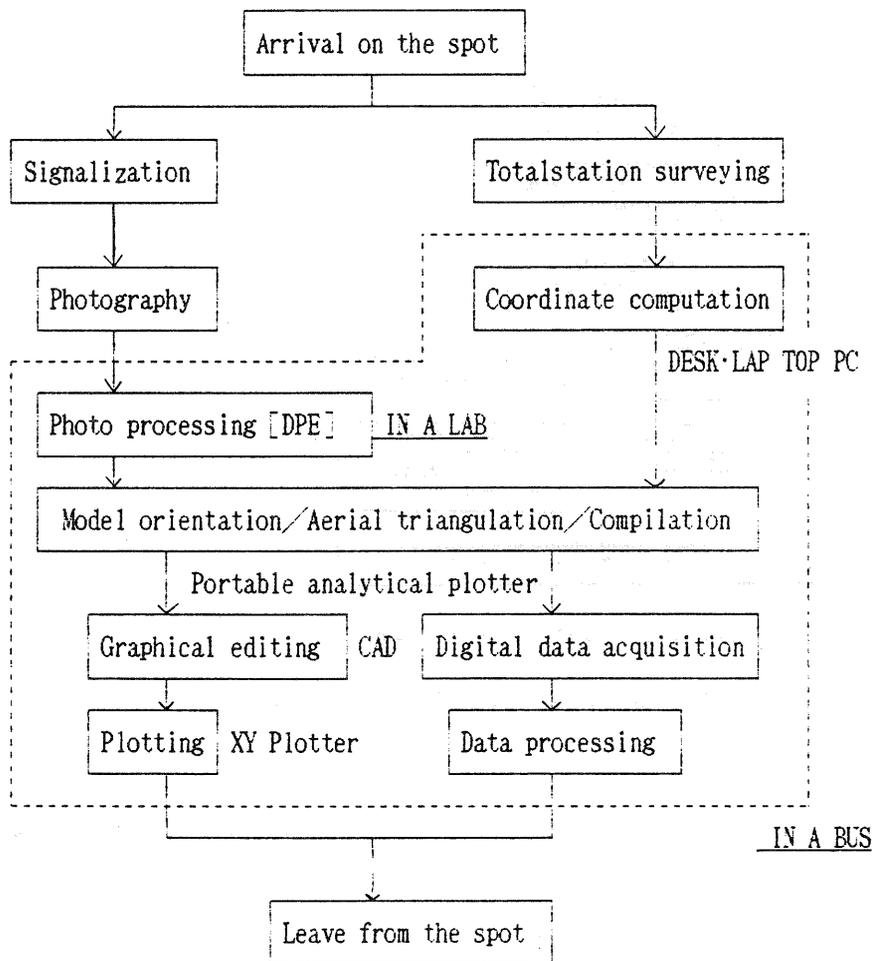
Fig.4 Automobile method flow-chart
