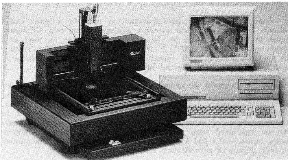
Fig. 2: Digital mono-comparator Rolleimetric RS1
