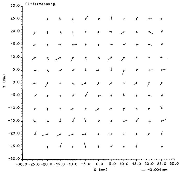
Fig. 5: Measurement of a calibrated grid plate
