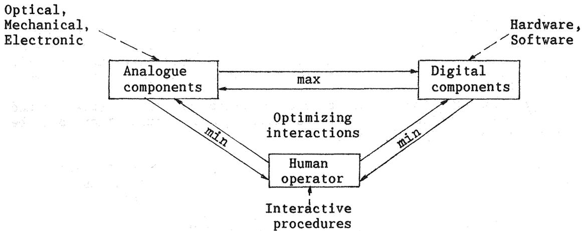
Fig. 5: Interfaces in a system
