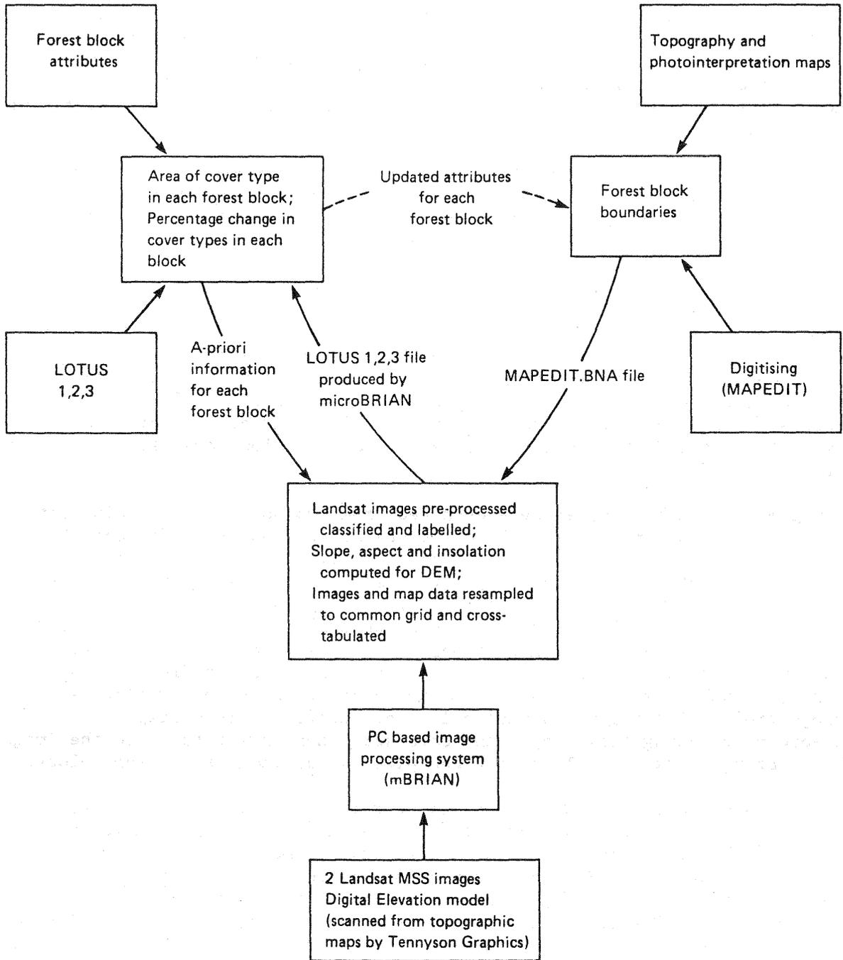
Fig. 2. GIS framework for example application.
