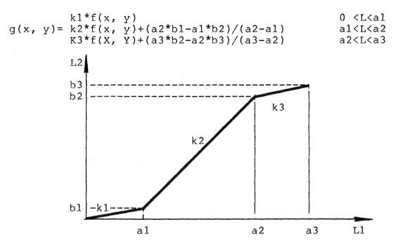
Fig. 2. Piecewise linear stretching
