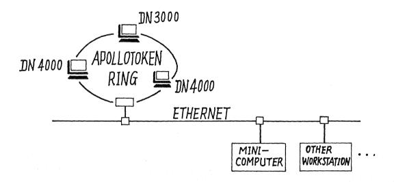
figure 1,2 distributed hardware configuration
