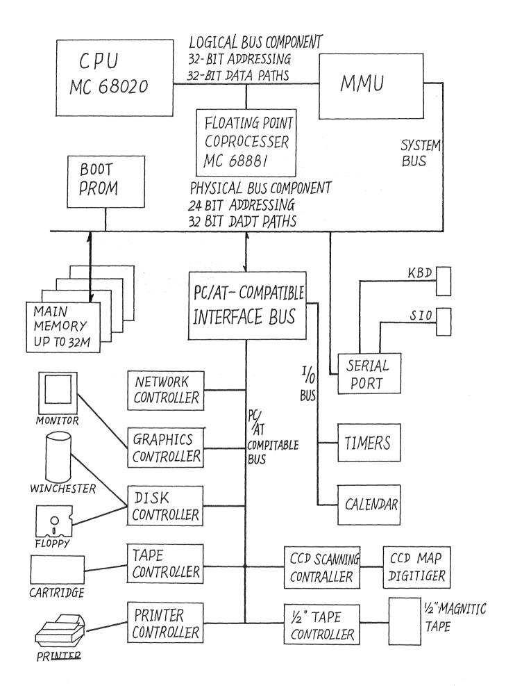
figure 1,1 hardware configuration(one workstation)
