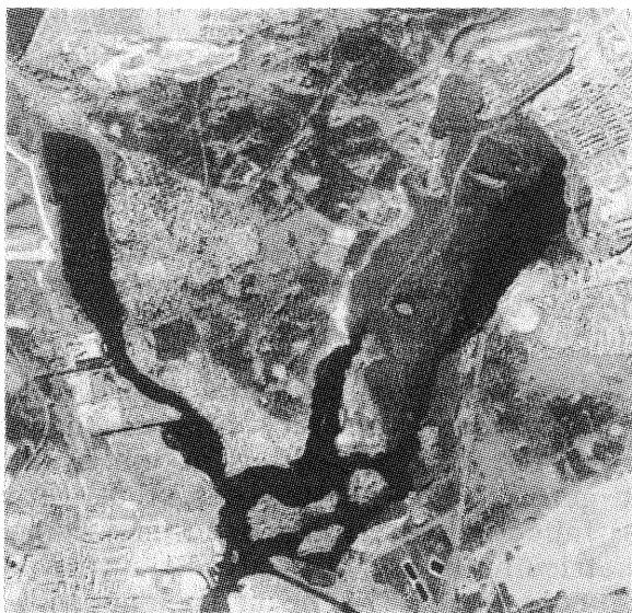
Fig.8 Destriped image from figure 6 after filtering in the spatial frequency domain
