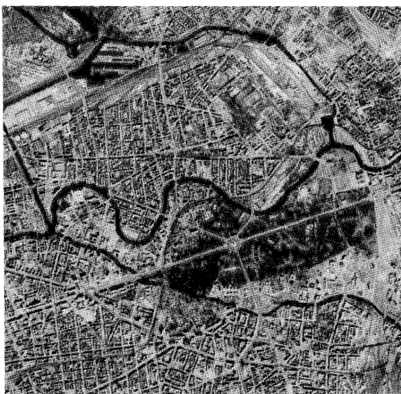
Fig.11: Enhanced red component after merging TM-band 3 and SPOT-HRV from figure 9 and 10
