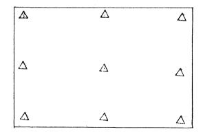
LMK AERIAL CAMERA with compensation of linear image motion is used. Photo scale is 1:11000. The focal length of photo camera  $f_k = 152$ mm. The fore-and-aft overlap is 60%. The lateral overlap is 55%. Whole test area has 11 strips. All control points are marked. The photo coordinate are taken on the PSK-2 Comparator. The results of block are:  $M_c = 0.18m$ . It can be met the requirment for the lower class network of coal mine.
