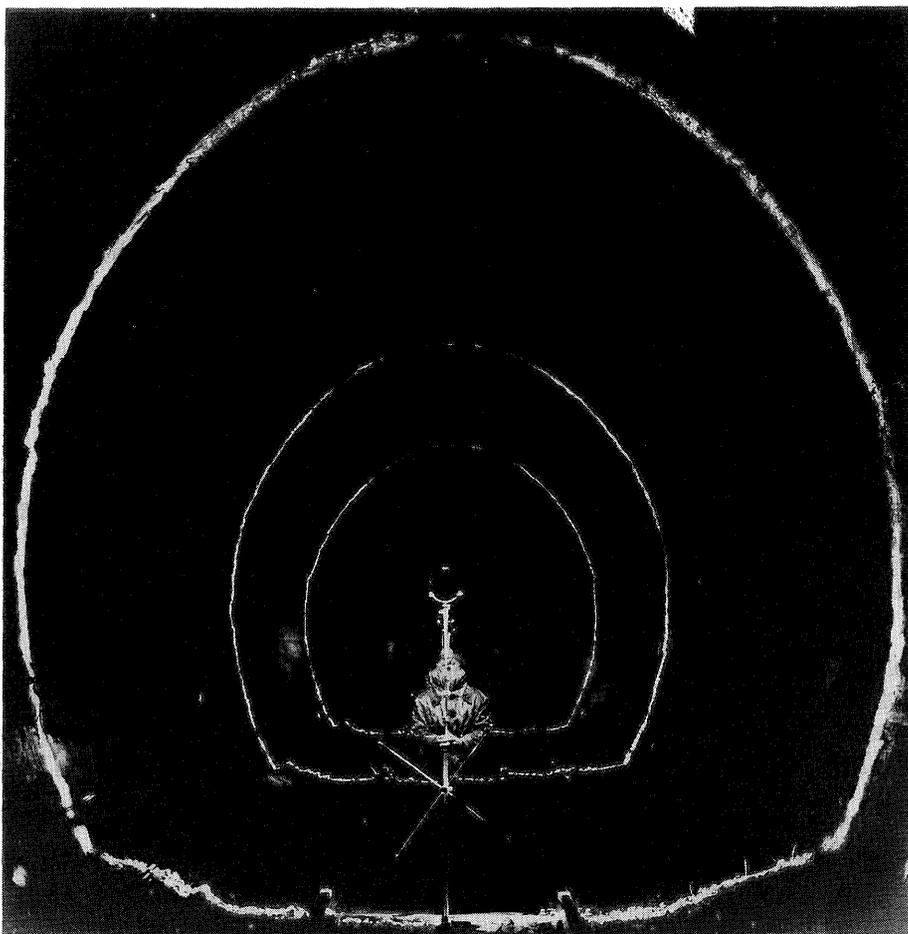
Figure 4 Contour recording on a WD plate
