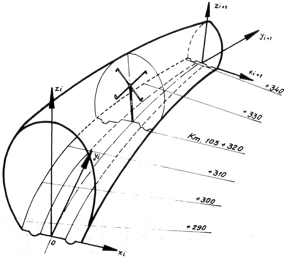
Figure 1 The scheme of the system of coordinates in the tunnel
