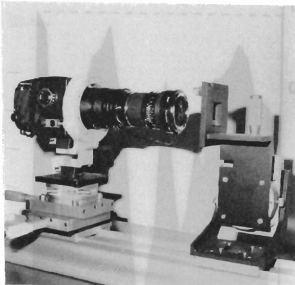
Fig.10 Bench mounting for photographing the small sandstone platen (Rolleiflex 6006 Réseau with extension tubes and retro-adapter)
