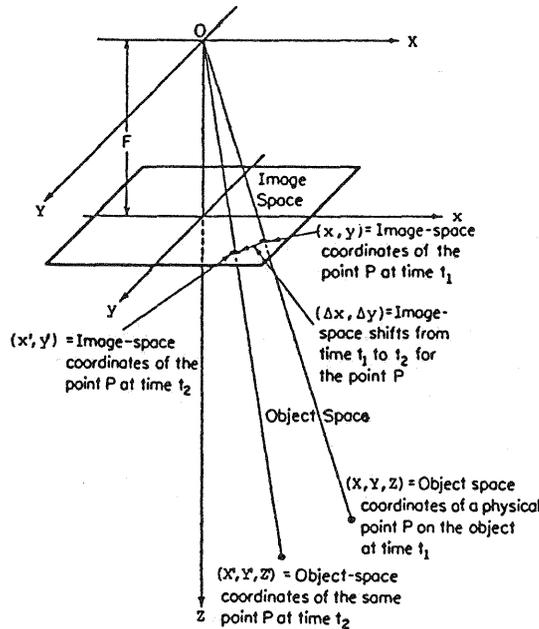
Fig.2: Basic geometry in 3-D motion estimation
