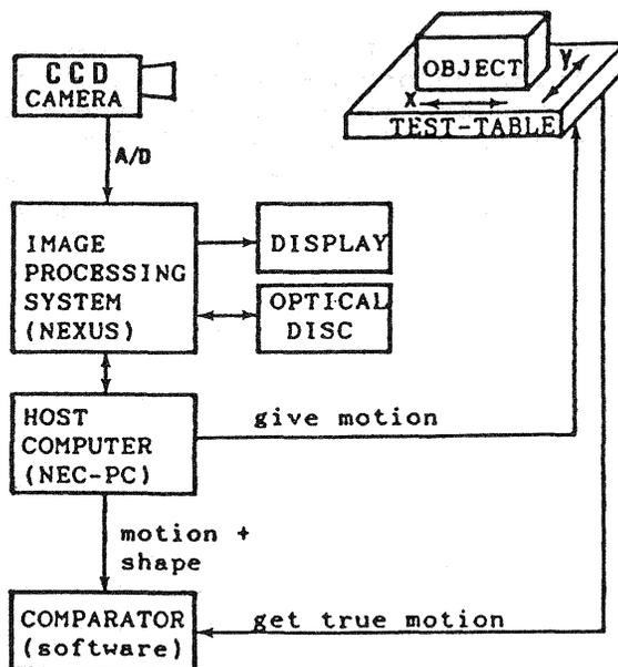
Fig.3: Experimental system for verifiable experiments in motion analysis
