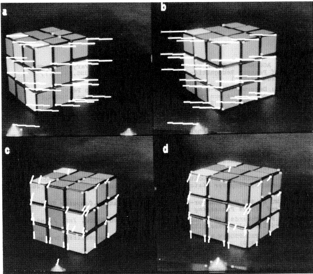
Fig.4: Two sequences with detected corner points and its displacement vectors; a) translation time  $t_1$ , b) translation time  $t_2$ , c) rotation time  $t_1$ , d) rotation time  $t_2$ .
